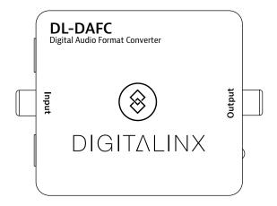
The DigitaLinx DL-DAFC is a Digital Coaxial / Optical audio converter. The DL-DAFC supports S/PDIF audio signal input through either Digital Coaxial or Optical cable and passes the signal (as is) to both Digital Coaxial and Optical output ports. With the DL-DAFC built-in amplification feature, it can serve as a repeater of the audio signal and extend the transferring distance.
