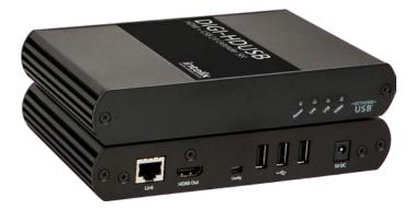
The Intelix DIGI-HDUSB extends HDMI and computer USB 2.0 signals up to 100m (330 ft) over twisted pair cabling. The DIGI-HDUSB 3-port USB/Video extender system supports full uncompressed HD video and USB 2.0 (up to 30Mbps) suitable for video applications in conjunction with keyboards, mice, and USB 1.1 web cameras. The DIGI-HDUSB supports HDMI video features such as 1080p, 4K, Deep Color and CEC/HDCP pass-through. The DIGI-HDUSB supports both USB 1.1 and 2.0 devices.
