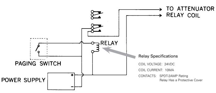
Power Switching Req. For - Pa Attenuators
