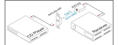
Example System: An AVO-A2-WP-F balun and AVO-A2-F balun connect a remote CD player to a receiver. The distance between these devices may be up to 2,500 feet. Two patch cords with RCA connectors are required to connect the baluns to the source and destination devices.
