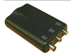
The Intelix AVO-V1A2 transmits a composite video signal and two analog audio signals up to 2,200 feet over structured cabling, such as Cat 5. Used in pairs, AVO-V1A2 baluns replace bulky coaxial cable and utilize a building's existing Cat 5/LAN cabling.
