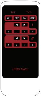
TV1, TV2: Turn on/off CEC enabled display device.
