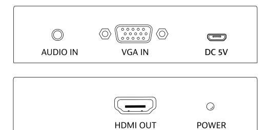
The DigitaLinx DL-VHD is a VGA to HDMI converter that converts computer video and stereo audio to HDMI. The DL-VHD VGA input supports resolution up to 1920x1200@60Hz along with HDMI output support of HDMI 1.4. The DL-VHD features fixed EDID mode and superior ESD protection. The DL-VHD is a Plug and Play device which allows for a hassle free install.
