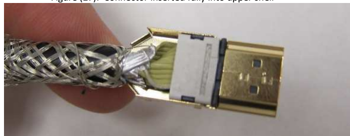
Figure (27): Connector inserted fully into upper shell
