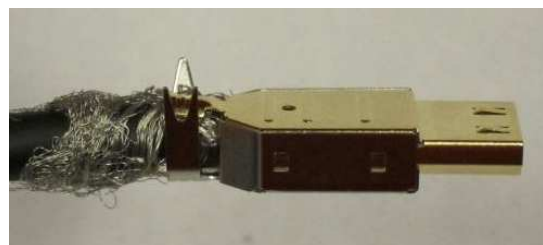
Figure (29): Properly assembled connector shells.
