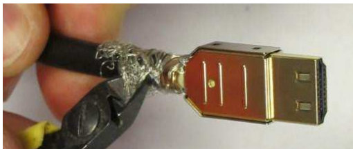
Figure (33): Trimming braid shield
