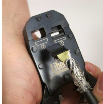
Figure (25): Assembled connector into Slot 2
