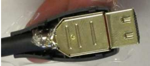
Figure (35): Assembled Connector laid into lower hood.
