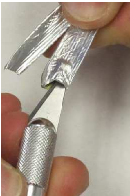
Figure (11): Separating the Ribbon Cable From the shield
