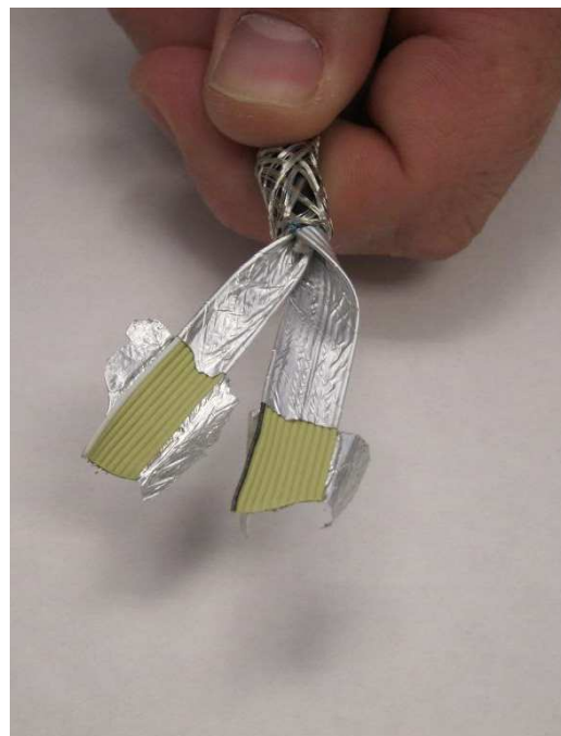
Figure (12): Partially removed foil shield
