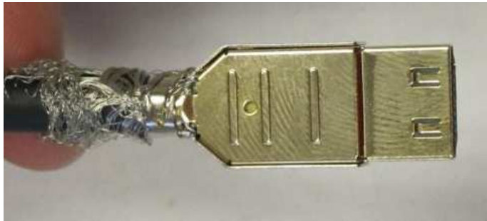
Figure (32): Properly crimped strain relief
