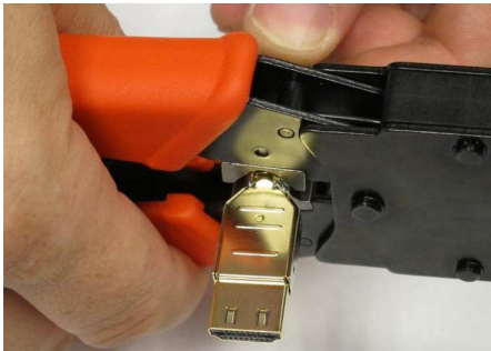
Figure (31): Strain Relief Crimp
