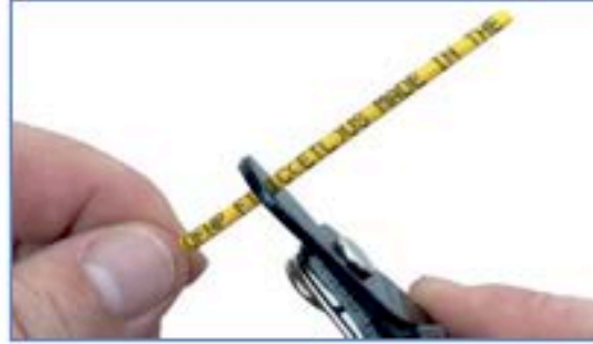
Step 2: strip back 50mm (2 inches) of the outer jacket
