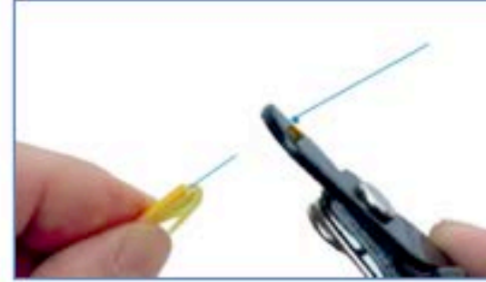
Step 3: separate the yarn from the fiber and use your three-hole stripper to remove the inner coating
