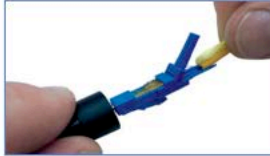
Step 6: insert the fiber into the connector and slide the locking tab closed
