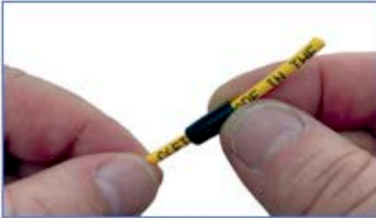
Step 1: slide the connector boot onto the fiber
