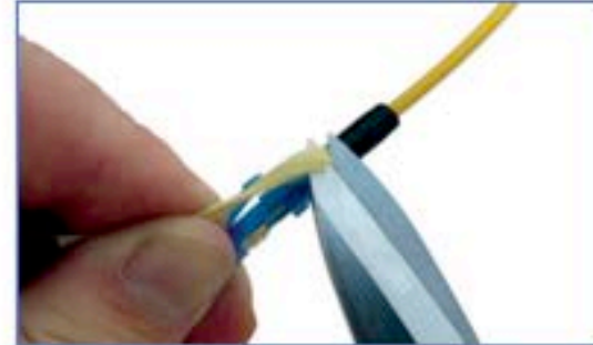
Step 7: screw the connector boot onto the connector, slide on the dust cap, and trim the exposed yarn
