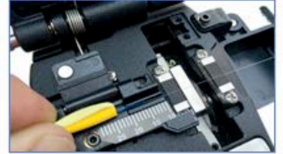
Step 4: cleave the fiber to length (28mm for SC connectors / 24mm for LC connectors)
