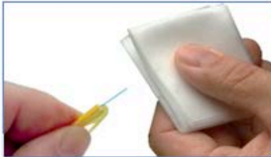
Step 5: clean any impurities from the fiber strand using an alcohol wipe
