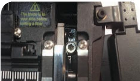
5. Attempt to cleave NSF fiber. If the fiber does not successfully cleave repeat Blade UP steps A & B to increase blade height until a successful cleave is achieved, reassemble.
