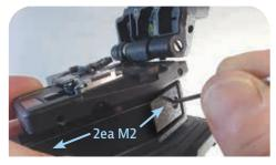
**2.** Using the M2 Allen wrench remove the two screws that secure the guide cover.
