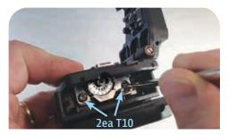
Loosen the two T10 guide screws with the supplied wrench. Approximately one turn is required. Do not loosen completely.
