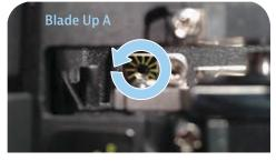
A. Loosen the T10 hex screw located behind the blade; looking down on the unit, turn counter clockwise one full turn.
