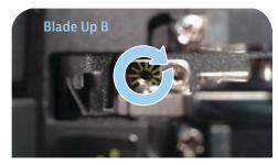
**B.** Turn the M2 Allen screw clockwise two positions. Tighten the previously loosened T10 hex screw and the two T10 side guide screws clockwise until snug.
