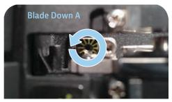
A. Loosen the T10 hex screw located behind the blade; looking down on the unit, turn counter clockwise one full turn.
