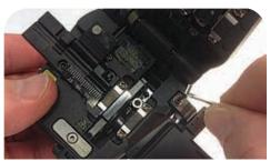
**1.** Using the M2 Allen wrench included with the cleaver, on the top right side remove the screw that secures the fiber scrap box. Set the scrap box aside.
