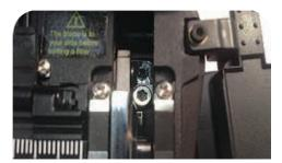
Attempt to cleave NSF fiber. If the fiber does not successfully cleave repeat Blade UP steps A & B to increase blade height until a successful cleave is achieved, reassemble.
