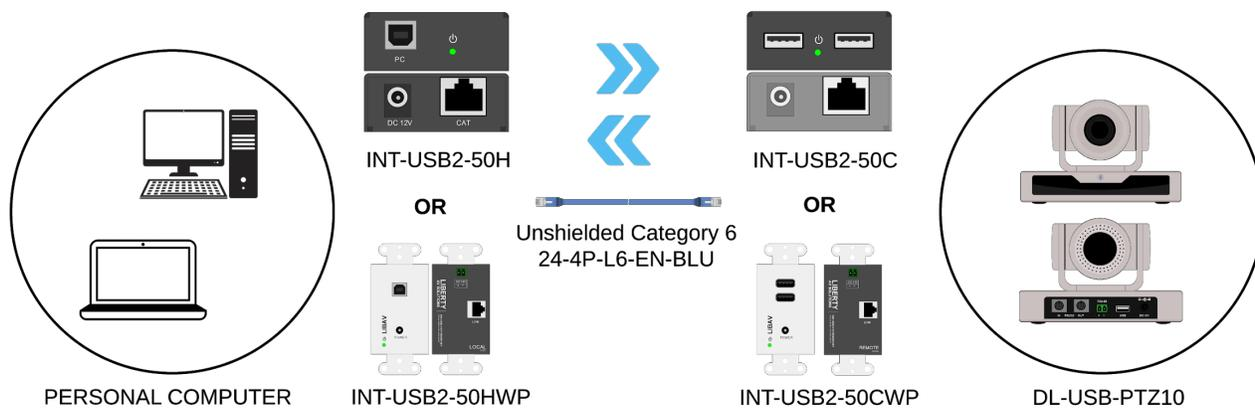
\*Camera external power supply is optional when using certified Liberty extenders and cable.
