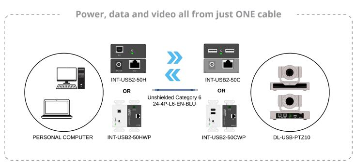
\*Camera external power supply is optional when using certified Liberty extenders and cable.
