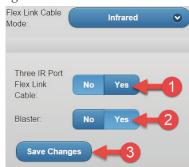
To use the Blaster cable with the Flex Link Triport cable, plug it into the port labeled 3, then change the Three IR Port Flex Link Cable setting to Yes. Then change the Blaster setting to Yes, and select Save Changes to apply the new settings.
