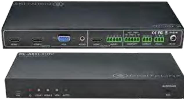
The **DL-AS31-2H1V** is a multiformat auto-switcher with two HDMI inputs and one VGA with analog audio input, one HDMI output, and one balanced analog audio output. This auto-switcher supports HDMI resolutions up to 4Kx2K at 30 Hz and multichannel audio and VGA video resolutions up to 1920x1200 at 60 Hz. In addition to passing EDID information from the display, there are multiple built-in EDID settings to simplify an installation.
