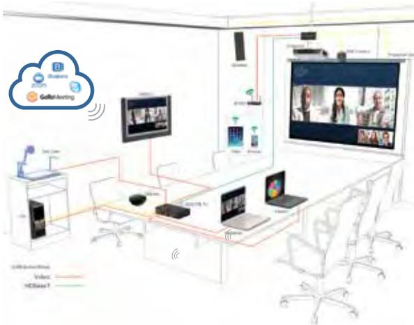
Input on RX allows you to incorporate wireless gateways to wirelessly screen share! System automation built in! It automatically powers up TV or projector via RS232, up/ down relays for projector screens with no need for separate system control.
