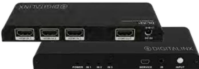
The DigitalInx DL-A31 is a three input by one output slim HDMI matrix with Ultra HD 4K support. The DL-A31 is HDMI 2.0, HDCP 2.2, and DVI 1.0 compliant. The matrix switcher offers video formats such as 4K/30Hz with 24bit at 4:4:4/ 4:2:2 and up to 4K/60Hz with 12bit at 4:2:0. The DL-A31 can be controlled via IR Remote or front panel.
