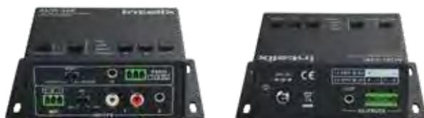
The Intelix **AUD-220** is a 2x20 watt Class D amplifier with 8Ω speaker output. The amplifier features two analog audio inputs and a balanced microphone input with ducking functions. Additional features of the AUD-220 include input and microphone volume control, bass and treble adjustments, microphone mixing with source audio, and three modes of microphone input support (48 dB gain, 48 dB gain with 48V phantom power, and line level).
