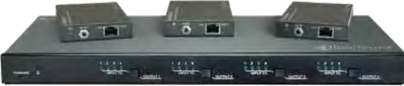
The **DL-44E-KIT** is a professional 4K HDBaseT Home Distribution Hub Kit, which consists of a 4K HDBaseT Matrix Switcher, 3 HDBaseT Receivers and accessories. The DL-44E-KIT is a professional 4x4 HDBaseT Matrix Switcher that consist of the following inputs and outputs, 4 HDMI IN (4Kx2K@60Hz signal at max), 3 IR IN, 1 IR EYE, 4 IR OUT, 3 HDBaseT OUT, 1 HDMI OUT, 1 SPDIF OUT, 1 L&R RCA OUT, and TCP/IP, RS232 control port via phoenix connector.
