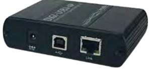
The Intelix **DIGI-USB2-4P** extends computer USB 1.1 signals up to 100m (330ft) over twisted pair cabling to four remote devices. The DIGI-USB2-4P utilizes inexpensive twisted pair cabling & has a throughput of up to 480Mbps.
