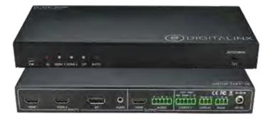
The **DL-AS31-2H1DP** is a multiformat autoswitcher with two HDMI inputs and one DisplayPort with analog audio input, one HDMI output, and one balanced analog audio output. This auto-switcher supports HDMI and DisplayPort video resolutions up to 4Kx2K at 30 Hz and multichannel audio. In addition to passing EDID information from the display, there are multiple built-in EDID settings to simplify an installation.
