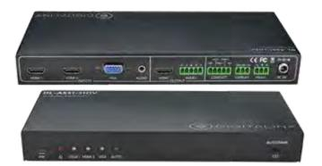
The **DL-AS31-2H1V** is a multiformat autoswitcher with two HDMI inputs and one VGA with analog audio input, one HDMI output, and one balanced analog audio output. This auto-switcher supports HDMI resolutions up to 4Kx2K at 30 Hz and multichannel audio and VGA video resolutions up to 1920x1200 at 60 Hz. In addition to passing EDID information from the display, there are multiple built-in EDID settings to simplify an installation.
