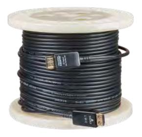
The **DL-PHDM-M-\*\*\*M** extends HDCP compliant HDMI® signals via a flexible, plenum rated, Active Optical hybrid cable assembly. Utilizing active circuitry in the permanent HDMI connectors, HDMI signals with video resolutions up to 4K@60Hz (18.0Gbps) can be transmitted on fixed length cables ranging from 10 meters up to 100 meters. The HDMI to optical conversion circuits draw 0.07 watts of power, which is provided by pin 18 of the HDMI ports on the connected devices.
