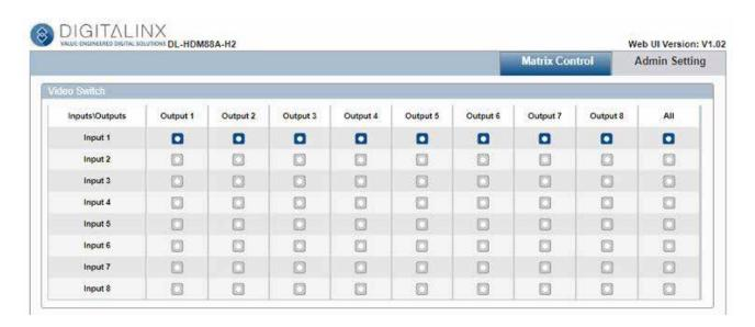
By default the audio switching routes follows video, in order to change this option in the matrix control so audio can be routed independently, change the *Independent switch mode* underneath the audio switch matrix to *Independent*. Routing audio in the matrix control will function the same as the video control above.
