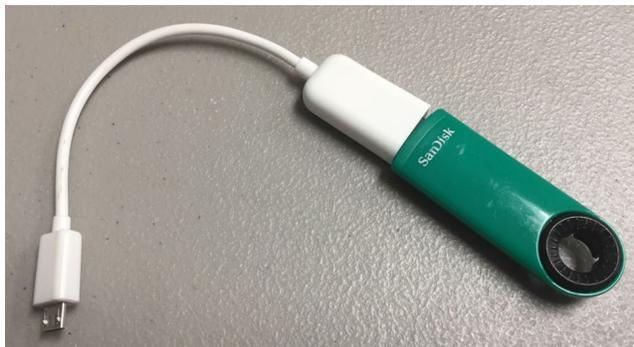
**STEP 4:** Connect the USB adapter to the FIRMWARE port of the AS-1H1V device
