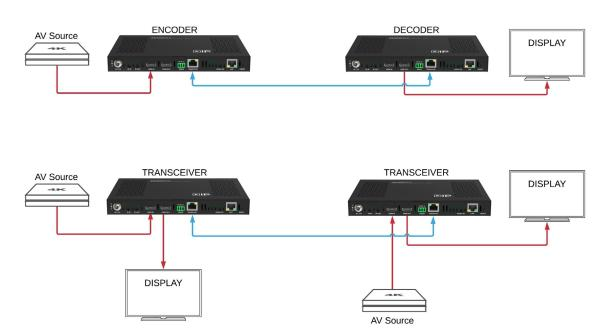
**Note:** Both transceivers must be connected to local power AC outlet with the supplied DC power supplies, the point to point application does not support PoE.
