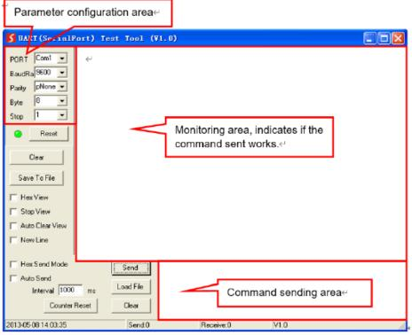
Please set the parameters of COM number, baud rate, data bit, stop bit and the parity bit correctly, then the RS232 commands can be sent in Command Sending Area.
